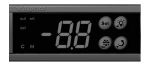
Working indicator: on-working; blinking-delay; off-stop. Setting indicator: on-setting status; blinking-defrost.
