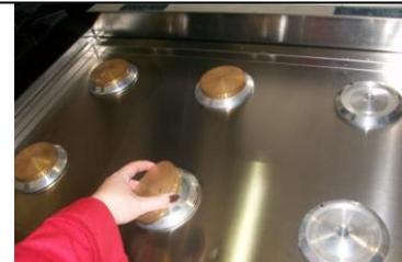
Lift off aluminium burner plates.
