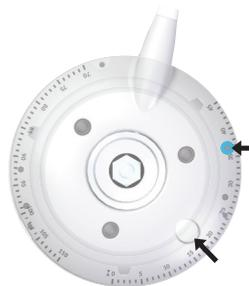
For the models with the micrometric *Parallel* system, first make sure that the grind point lock screw (7) is lined up with the locking foot. This will ensure that the lock screw and locking foot move in conjunction with one another, and that the locking mechanism works properly (Fig. 11).
