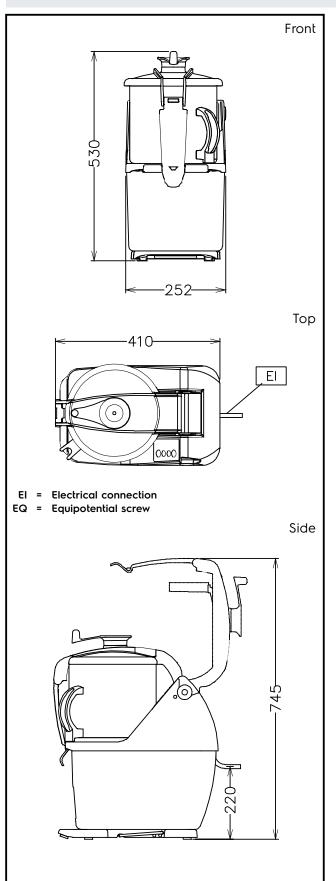
Electric Supply voltage: 603708 (TRK70VVEG) 200...240 V/1N ph/50/60 Hz Electrical power: 1.5 kW **Total Watts:** 1.5 kW Capacity Performance (up to): 550 - kg/hour Capacity 7 liter **Key Information** External dimensions, Height 530 mm
