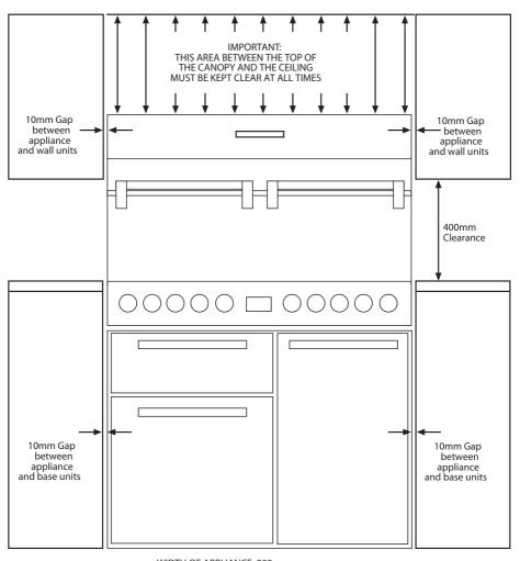
WIDTH OF APPLIANCE: 900mm HEIGHT OF APPLIANCE: 1520-1550mm
