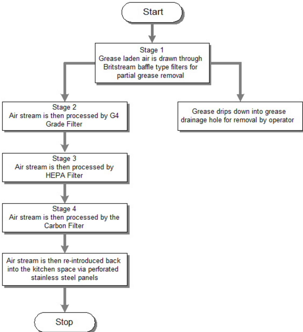
**Grease Drainage Hole:** Collected grease and moisture drains down and into the grease drainage hole. Refer to the picture below.
