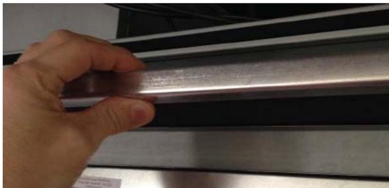
***Removing Each of the Stage 4 Carbon Filters***
