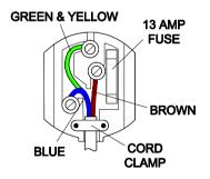
As the colours of the wires in the mains lead of your appliance may not correspond with the coloured marking identifying the terminals in your plug, proceed as follows:
