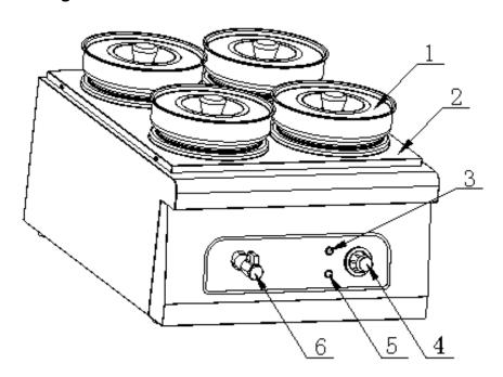
1---soup barrel2----furnace body3----power indicator4---thermostat5---heating indicator6---water outlet valve
