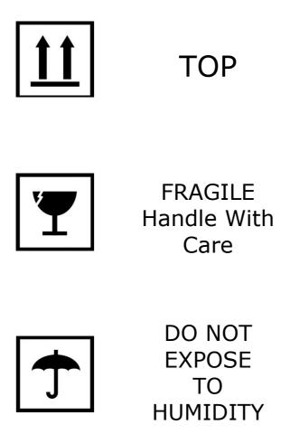
Units should be stored in an enclosed dry place and be protected from dust and dirt by means of a dust sheet, bubble wrap, cardboard or similar. All precautions must be taken to prevent the ingress of water into the unit or it's packaging
