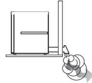
2. Use a 4" diameter rigid metal duct. Tape all joints, including at the dryer. Never use lint-trapping screws.
