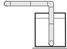
4. Clean all old ducts before installing your new dryer. Be sure the vent flap opens and closes freely. Inspect and clean the exhaust system annually.
