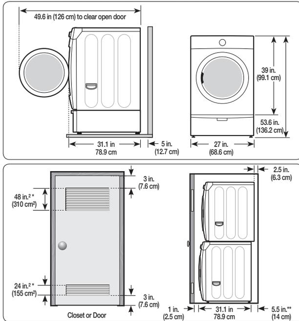
Required Dimensions for Installation With Stacking Kit
