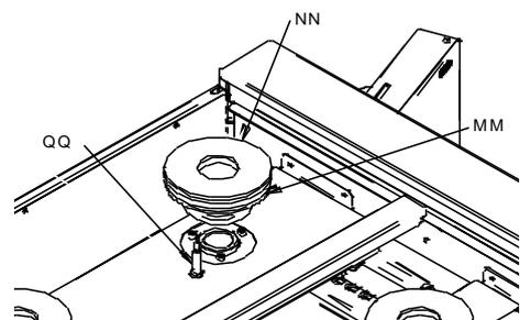
The Burner Body & Cap can be cleaned with a mild detergent and hot water solution using a soft bristled brush. Rinse and dry thoroughly with a dry cloth.
