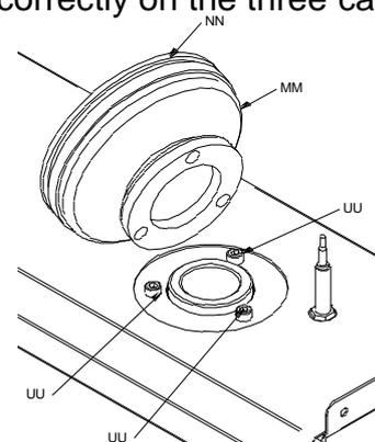
Pan Support Channel – Remove from the appliance taking note of its fixing points.
