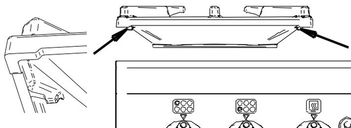
The Pan Supports can be cleaned with a mild detergent and hot water solution using a soft bristled brush. Rinse and dry thoroughly with a dry cloth.
