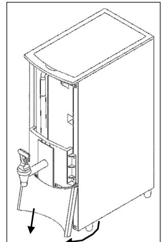
5. To remove the lower front panel, rotate the bottom of the panel forwards and slide downwards.
