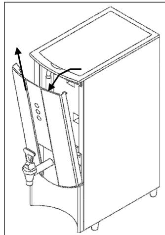
6. To remove the upper front panel, rotate the top of the panel forward and lift.
