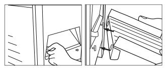
Fit the rear cover in the sloping/open position, resting on two locating pins.
