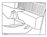
The control panel cover can then be attached to prevent further adjustment.
