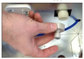
The blue pipe connects to the grey fitting which can be found underneath the appliance. The grey fitting can be unscrewed, and the blue pipe slots into it. Then screws back onto the appliance.
