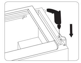
4. Reverse the door and mount it onto the left lower hinge.
