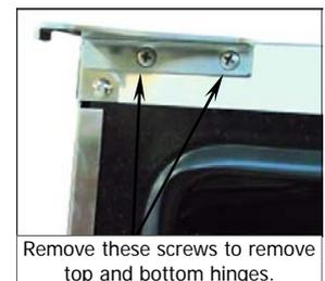
16. Remove Hinge Plate from bottom of oven and fit diagonally opposite, to upper corner.
