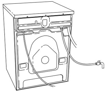
The water pressure must be 0.1–1 MPa (about 1–10 kp/cm<sup>2</sup>; 10–100 N/cm<sup>2</sup>).
