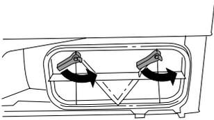
4. Take out the condenser and wash the fins using a hand shower. Do not poke anything into the gaps between the fins as this could damage the condenser. Do not use any sharp metal objects when cleaning.
