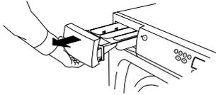
Then lift it upwards and outwards as shown.
