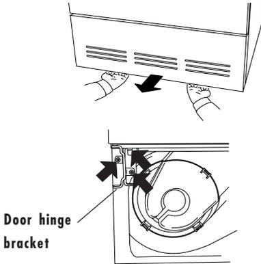
2. Pull the bottom edge of the door outwards while twisting the hinge bracket in the direction shown by the arrows.
