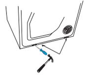
6. Slide the tumble dryer under the metal brackets, keeping the front edge raised 1–2 cm.
