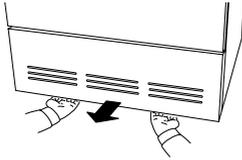
3. Open the cover over the condenser by turning the two levers anti-clockwise.
