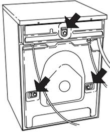
1. First unscrew the screw and remove the washer.
