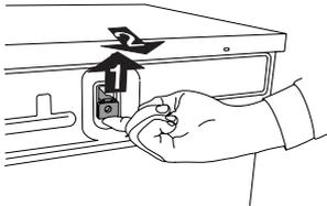
3. Finally, refit the rubber spacers to cover the transit holes.
