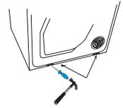
6. Slide the tumble dryer under the metal brackets, keeping the front edge raised 1–2 cm.
