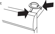
5. Open the knock-out holes on the back of the tumble dryer (where present) with the aid of a hammer and screwdriver. They must not be fully removed, just opened!
