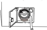
5. Remove any objects and waste from the pump housing. Check that the pump impeller at the back rotates freely.
