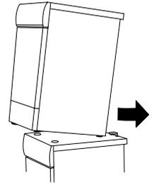
7. Lower the front feet of the dryer into the plastic cups and adjust the feet so that the dryer is level.
