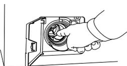
6. Screw the cap and trap back into place, reconnect the drain hose and close the flap.
