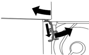
3. Move the hinge pin to the other side of the bracket. When the door is hung on the right side the hinge bracket must be turned upside down.
