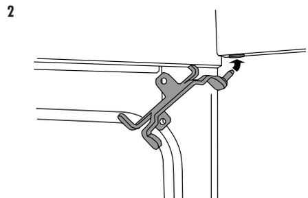
13. Fit the hinge bracket, tightening the screws in the order shown.
