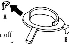
4. Position the plastic cups so that the arrowed lugs are flush with the front and side of the top, then press down onto the top. Now break off the remaining tabs.
