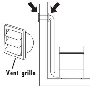
If there is only one vent duct from the room then a vent spacer must be fitted.
