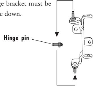
4. Then transfer the hinge pin in the underside of the top panel to the right side.
