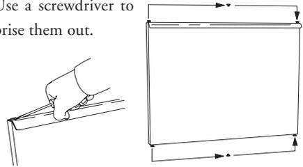
6. Unscrew the two screws from the edges of the door about five millimetres so that you can remove the door magnet and plate from the inside of the door.
