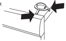
5. Open the knock-out holes on the back of the tumble dryer (where present) with the aid of a hammer and screwdriver. They must not be fully removed, just opened!
