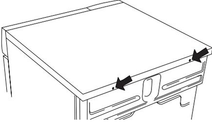
2. Fit the metal brackets as shown, using the screws.
