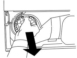
6. Refit the fan and tighten the nut.
