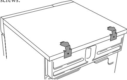
3. The plastic cups that will hold the front feet of the tumble dryer must be attached to the top of the washing machine. This is important since the feet of the tumble dryer must be located in the plastic cups to ensure that the dryer is correctly positioned.
