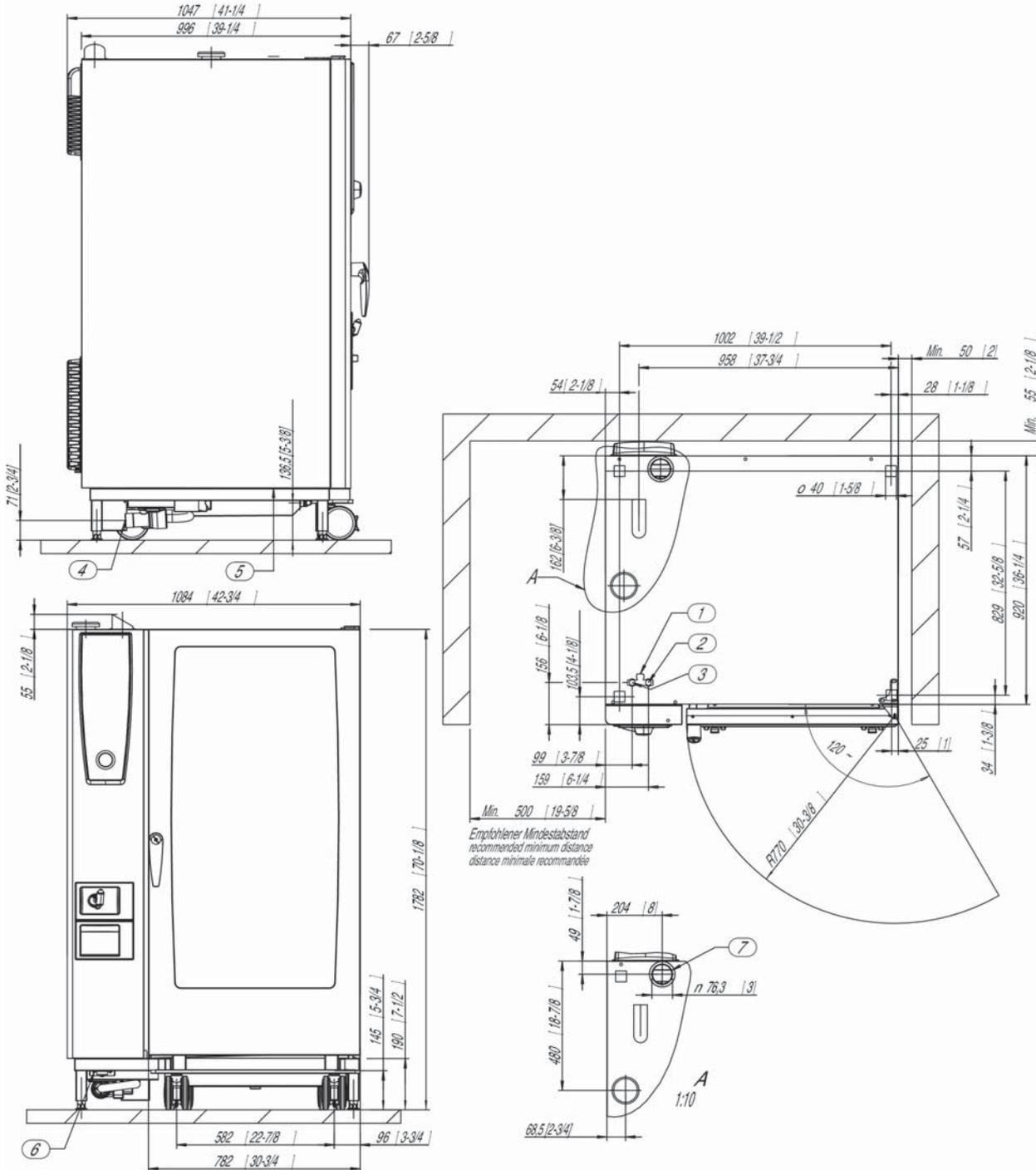
1. Common water supply (cold water) "Single" water connection as shipped 2. Water supply cold water / condensate "Split" water connection 3. Water supply cold / Treated "Split" water connection 4. Water drain 5. Electrical connection wire entrance 6. Chassis Ground connection 7. Steam Vent pipe DN 3" / 78 mm minimum distance 2" / 50 mm Measurements in mm (inch)
