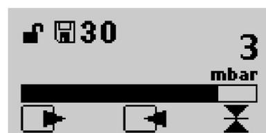
Fig. 23: Sealing status display (050)
