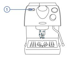
1. Remove the filter holder from the group and press the brew start/stop button and allow water to flow from the group for about 10seconds, press the brew start/stop button to stop the flow. Use a shower plate brush (Fracino part no. FC54) to dislodge dried coffee particles in the group and around the filter holder washer to prevent a build up of coffee.
