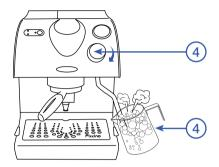
4. When the "tone" changes turn the steam off, as this is an indication that the milk is beginning to boil. If using a thermometer turn the steam off when the temperature is approaching 65-70°C. Taking the milk above this temperature will affect the texture and taste of the milk.
