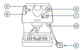
**8.** Wait for the steam to start venting from the steam tube this should take 2 or 3 minutes, then close the steam valve by turning the handle clockwise.
