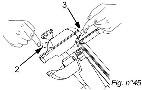
**N.B.:** Do not carry on the deburring operation for more than 3/4 sec. to avoid the damaging bending of the blade edge.
