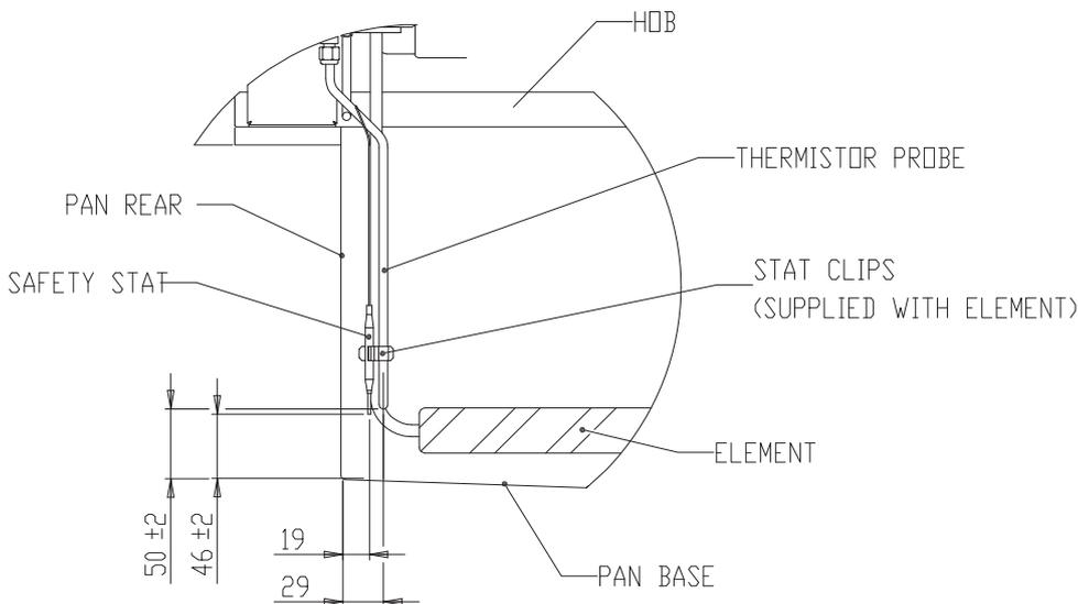
THERMISTOR PROBE AND SAFETY STAT BULB TO BE CLIPPED INTO POSITION AS INDICATED.
