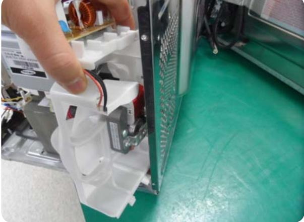
A photograph showing a person's hand removing a screw from the back panel of the chassis. The back panel is a green metal sheet, and the screw is being removed from a hole. The magnetron assembly is visible in the background.                        | <p>6. Remove two screws from the back panel.<br/>7. Take out the fan motor.</p> |
