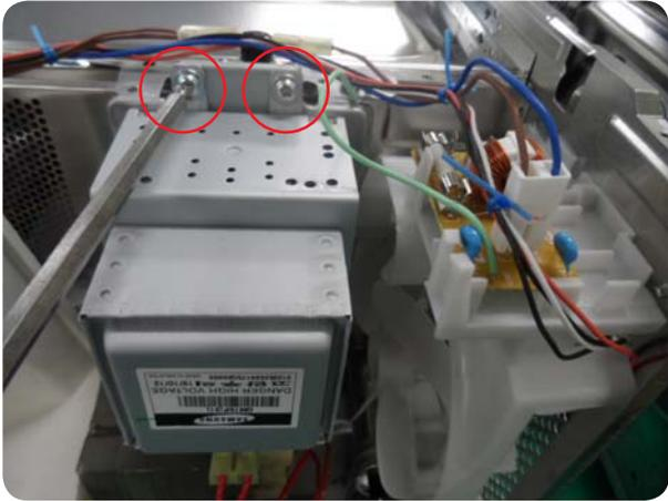
A close-up photograph of the magnetron assembly. Two screws on the top surface of the metal housing are circled in red. The assembly is connected to various colored wires (red, blue, green, yellow) and is mounted on a white plastic support structure. | <p>4. Remove screws securing the magnetron to the wave guide.</p>               |
