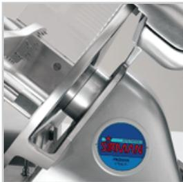
Remarkable clearance between blade and machine body
