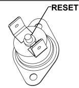
WARNING: IF THE THERMAL CUTOUT HAS TRIPPED, THE REASON FOR OVERHEATING MUST BE IDENTIFIED AND REMEDIED BEFORE PUTTING THE UNIT BACK INTO SERVICE.
