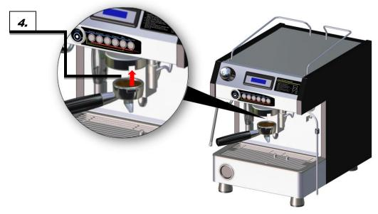
**5.** Firmly turn the filter holder anti-clockwise, until the handle of the filter holder is pointing towards you.
