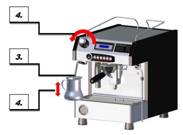
**5.** When the milk is at the required temperature (65-70°C) and consistency, close the steam valve.
