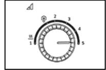
2. Set the desired heating time by rotating the **TIMER** knob.
