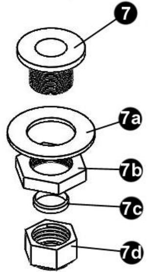
External Drain Tube Assembly
