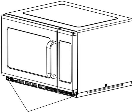
To restall,align the base plate mounting holes, clockwise the metal nails to tighten .
