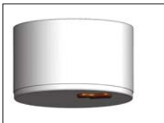
Figure 14 Excessive food spillage stuck to pan base will impinge the pan balance. One side of the utensil will be further away from the induction field than the other. This could reduce efficiency and it will also cook one side of the pan faster. Keep pans clean to ensure efficient cooking.
