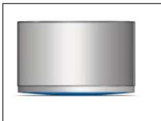
Figure 12 Pan base is bowed out and is NOT FLAT. The unit efficiency will be dramatically reduced during cooking. It may not even be detected by the appliance. Note: This is also liable to happen if pans are damaged, e.g. large dents.
