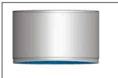
Figure 13 Pot base is bowed inward and is NOT FLAT; The unit efficiency will be dramatically reduced during cooking. It may not even be detected by the appliance. Note: This is also liable to happen if pans are damaged, e.g. large dents.
