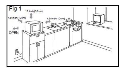
A 10-cm spacing should be kept between the appliance and right and back walls, and a 30-cm spacing kept on the top. Never dismantle the appliance's feet, nor block the air intake and exhaust opening. The left side must be open.
