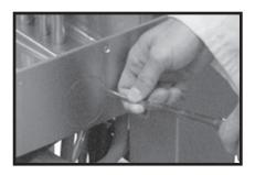
Break out perforated disk at the tank panel (either at the right or left side).
