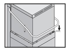
To avoid heat loss, lower hood to "Stand By" position between wash cycles.
