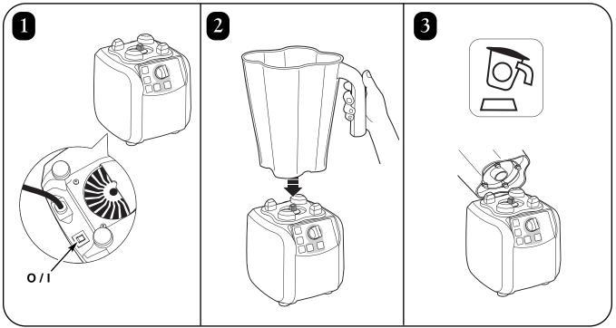
The location of the main power switch will be either on the front of the unit or on the bottom of the unit as indicated above. Jar pad sensor with four magnetic connections to prevent blending unless container is on correctly.
