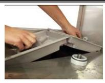
Re-mount all filters and drain plug (where applicable).
