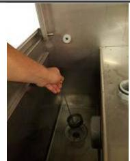
Remove and clean the secondary filter, located in bottom of wash cabinet. (*drain pump machines*)
