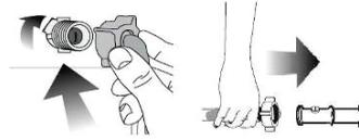
Ensure the rubber seals within the ends of the hose are in place.
