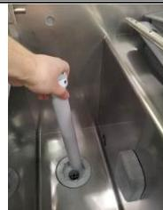
Remove the drain plug (*gravity drain machines*)
