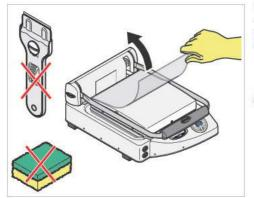
Slowly remove the protective films from the appliance: clean any glue residue with appropriate solvents without using tools, abrasive detergents or acids that could ruin the surfaces.
