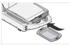
The supplied fat collection drawer to collect the liquid waste that is deposited on glass ceramic surfaces. The rounded drainage channel for the liquids, flowing all around the hobs, can easily convey liquids and dirt into the removable drawer to further facilitate the clearing. Before to use for the fist time the grill insert thesupplied fat collection drawer in the in the front seat as shown in the 'image.
