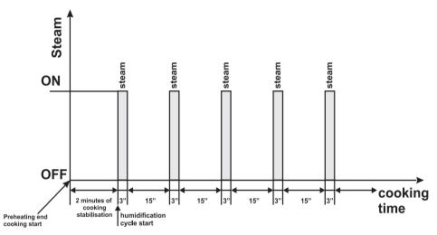
WARNING: the humidification cycle begins 2 minutes after cooking starts to allow complete stabilisation of the oven temperature.
