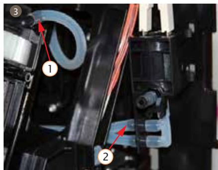
3. Pull out two silicon pipes from the left side of the machine
