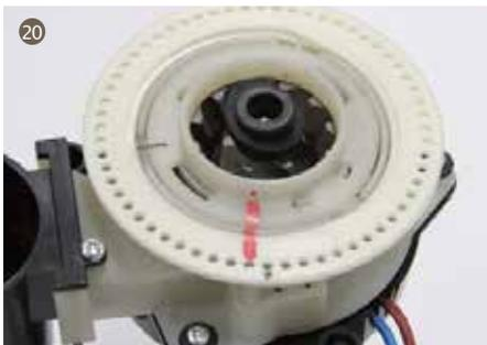
20. Insert the already installed upper burr into motor support for grinder, and adjust the gap between the conical burr and upper burr.
