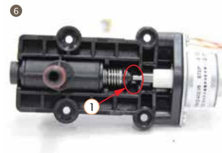
6. Rotate the tail of the stepper motor to make the axis of the stepper motor stand up to the drain valve support until it cannot stand up any more.
