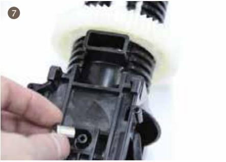
7. Rotate the gear onto the brew unit frame, install the sleeve pipe, the small head of sleeve pipe should be inward.
