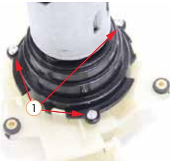
8. Install the coffee powder container into the gearbox, the bigger hook on the coffee powder container should compare to the bigger groove. Screw tightly.
