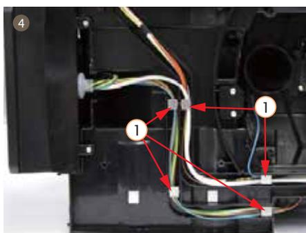
4. Disassemble 5 cable racks
