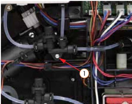
4. Disassemble 1 screw from dispenser valve 3W
