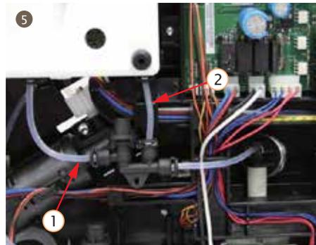
5. Pull out Teflon pipe which connected thermoblock group and dispenser valve 3W and dispenser valve 2W
