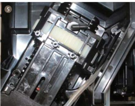
5. Pull the brewing unit outward and rotate the gear clockwise to the position as the picture shows
