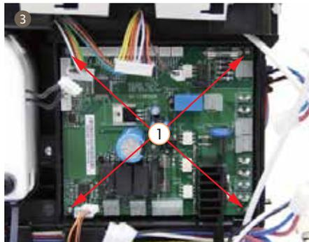
3. Disassemble 4 screws on PCBA, and take out PCBA
