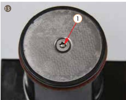
13. Disassemble the screw from contropistone, and take out filter screen
