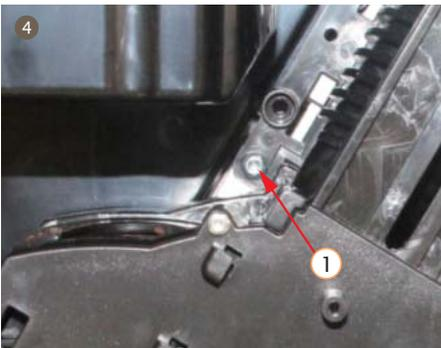
4. Disassemble 3 screws from brew unit
