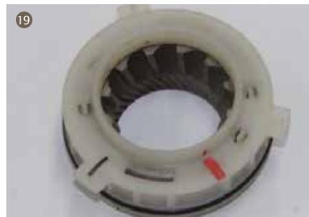
19. Assemble upper burr, upper grinder support, upper grinder cover and support seal together.
