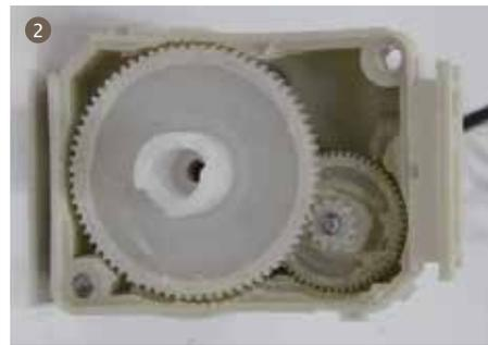
2. Install dispenser valve gear A and dispenser valve gear B into dispenser valve gearbox after coat oil(MI-setral-61B).
