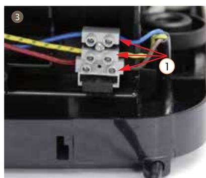
3. Disassemble 1 screw from support, loose 3 screws inside the line pencil connector and take out the power cord
