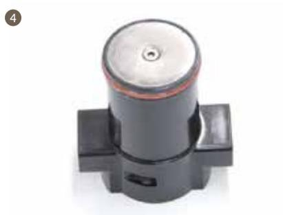
4. Coating the contropistone seal with lubricating oil (SYN-setral-AI/C 2-FD) and install to the contropistone, and then lock the filter screen.
