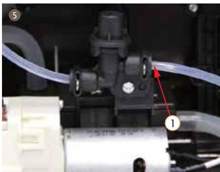
5. Pull out Teflon pipe between dispenser valve 2W and drainage valve
