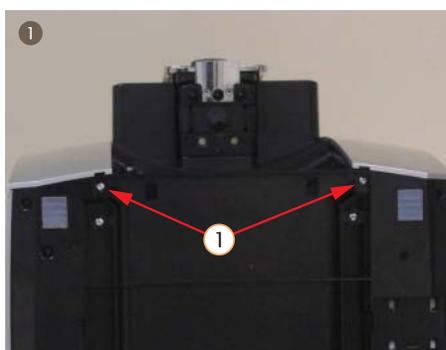
1. Disassemble the 2 screws from the bottom
