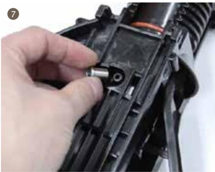
7. Take out left and right pull plate and pull plate sleeve
