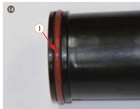
14. Disassemble seal from contropistone
