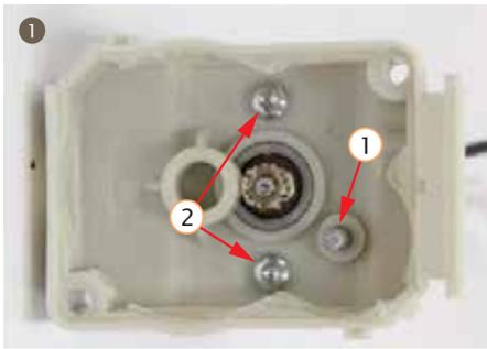
1. Press the gear pin into the hole of the gearbox, and put the dispenser valve motor to gearbox . The screws need a few loctite.
