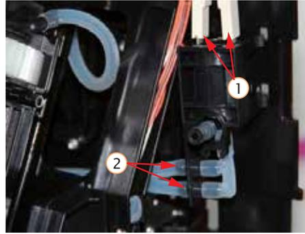
3. Pull out terminal and silicon pipe and take out solenoid valve group
