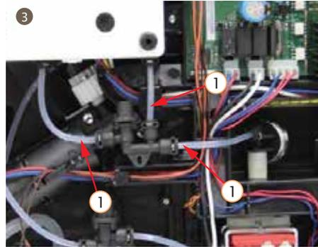
3. Pull out 3 Teflon pipes which connected to dispenser valve 3W, and take out dispenser valve 3W
