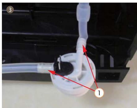
3. Pull out the silicone pipe at two sides of the flowmeter, and take out flowmeter
