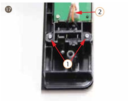
17. Take out 2 screws from the switch support, pull out the terminal from the HMI, and take out the switch group
