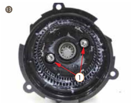
13. Disassemble the 2 screws inside the gearbox, and take out the grinder motor
