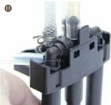
11. Pull out all the silicon pipes
