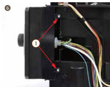
6. Disassemble 2 screws from the support
