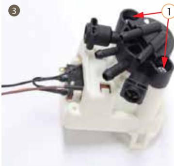
3. Disassemble the 2 screws from the dispenser valve
