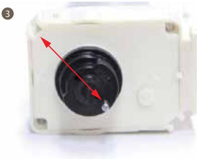
3. Install the gear box lid and sheave drive part, pay attention to the position of the sheave drive part.
