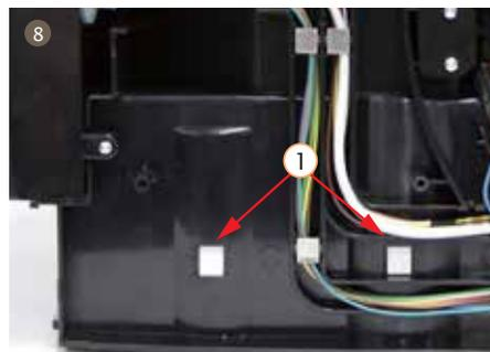
8. Disassemble hooks from the support and take out thermoblock
