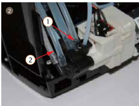
2. Pull out two silicon pipes from the dispenser valve on the right side of the machine
