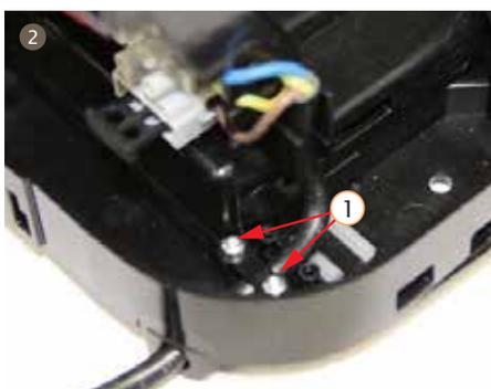
2. Disassemble 2 screws from the cable rack
