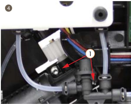
4. Disassemble 2 screws from support and take out geared motor group
