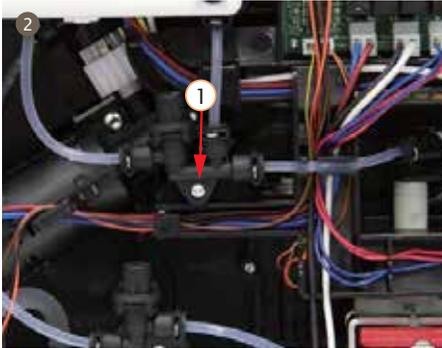
2. Disassemble 1 screw from dispenser valve 3W so that the wire can be taken out from the cable rack
