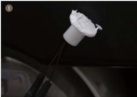
1. When install the NTC on the thermoblock, cover NTC with silicone grease and fasten it.
