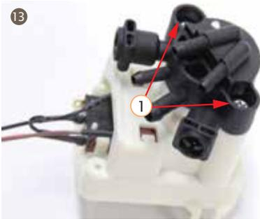
13. Assemble the water distributor to the dispenser valve, and lock the screws on both sides uniformly, the head of the screws need loctite.
