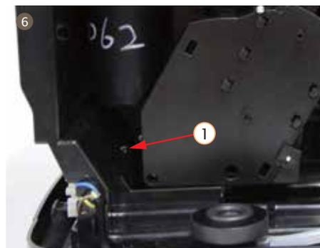
6. Disassemble 1 screw from backside and take out brew unit
