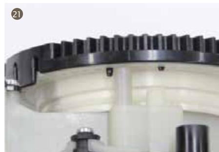
21. Install the grinder adjustment sensor to grinder adjustment ring. The position should be as the picture shows.
