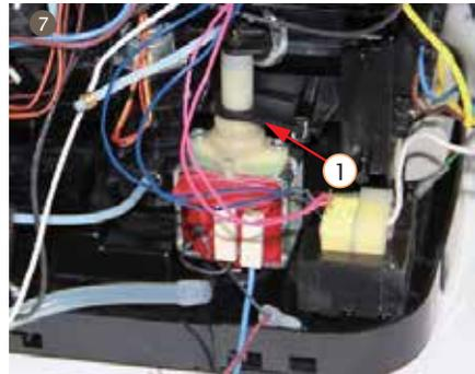
7. Pull out pump clamp from the support and take out pump group
