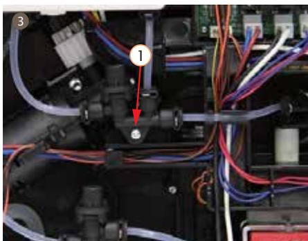
3. Disassemble 1 screw from dispenser valve 3W, so that the wire can be taken out from the cable rack
