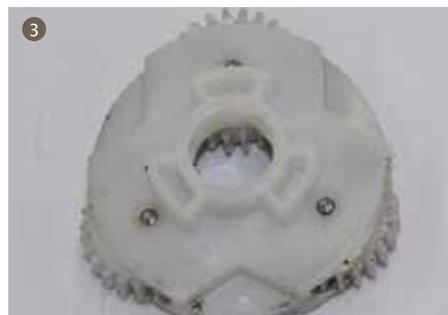
3. Install 3 epicyclic gear B and 3 epicyclic gear pin A into epicyclic gear support B, and coat with oil(MI-setral-61B).
