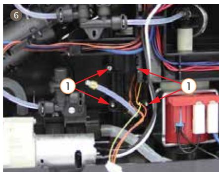
6. Disassemble 4 screws from support and take out drainage valve group
