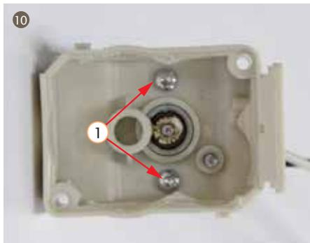
10. Disassemble 2 screws inside the gear box, and take out the motor for dispenser valve
