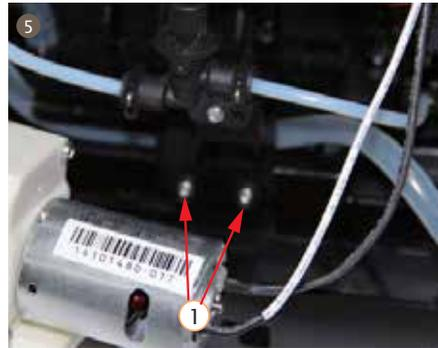
5. Pull out silicon pipe on condensator that connected to pump
