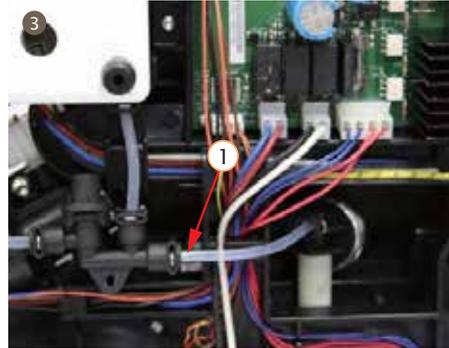
3. Pull out Teflon pipe on dispenser valve 3W that connected to pump
