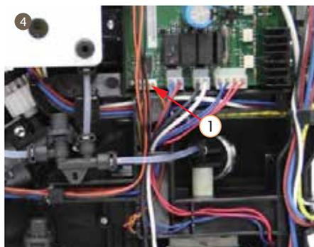
4. Pull out terminal from stepper motor on PCBA
