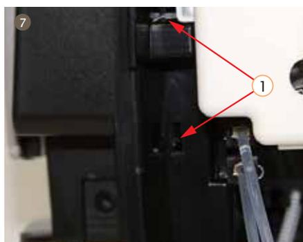
7. Disassemble left and right hooks on the support and take out control panel group
