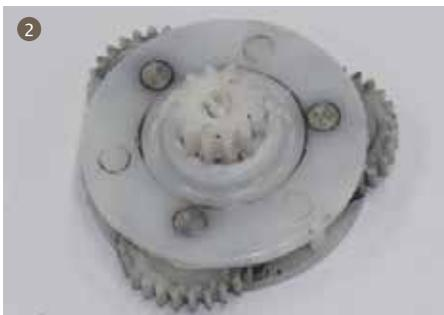
2. Install 3 epicyclic gear A and 3 epicyclic gear pin A into epicyclic gear support A, and coat with oil(MI-setral-61B).
