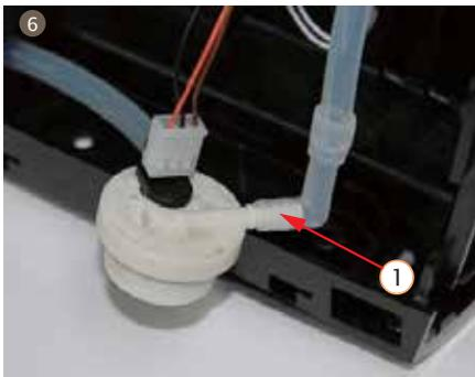
6. Pull out the flowmeter and pull out the silicone pip
