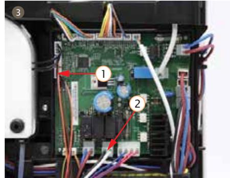
3. Pull out dispenser valve terminal on PCBA, and take it out from the cable rack
