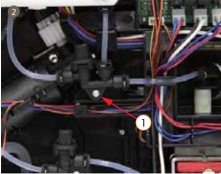
2. Disassemble 1 screw from dispenser valve 3W
