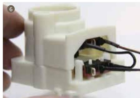
6. Assemble the sheave permanent seat and dispenser valve together.
