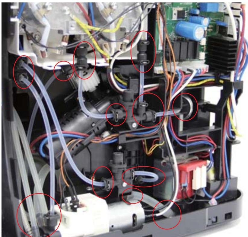
Check leakage of connectors
