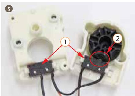
5. Install microswitch line pencil switches to sheave permanent seat and dispenser valve separately. Pay attention to the position and the direction of the sheave and microswitch.
