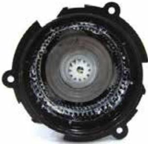
4. Put the already installed epicyclic gear frame A into the gearbox, put 1 filler piece onto epicyclic gear frame A.
