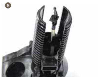
6. Assemble the already installed contropistone into the brew unit frame. Note: The direction of the contropistone should be the same as the picture showed.
