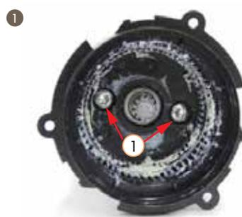
1. Assemble the grinder motor and gearbox together, and screw them tightly. The screw should be covered with loctite. The teeth of the gearbox should be coated with oil(MI-setral-61B). The red mark place should correspond to one hole of the gearbox.
