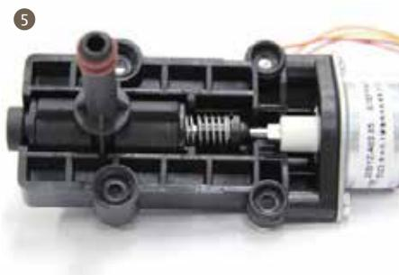
5. Assemble them into drainage valve, and install the seal, Teflon pipe and clamps.
