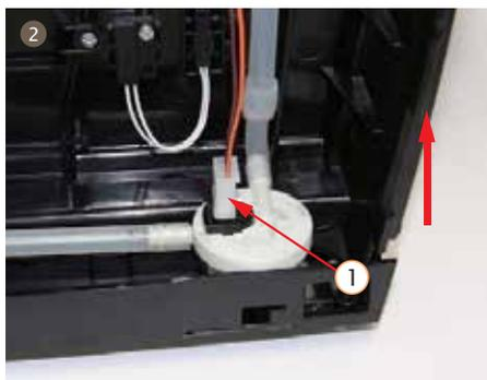
2. Pull out the flowmeter terminal, and pull out the flowmeter according to the arrow direction
