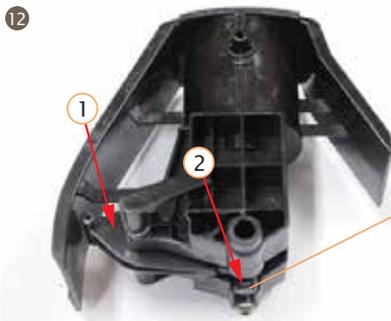
12. Disassemble release link, and take out piston
