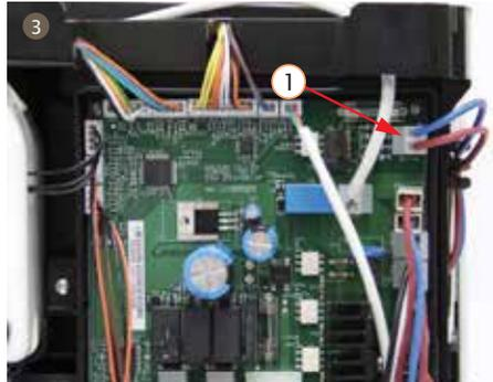
3. Pull out grinder motor terminal from PCBA and take out grinder group
