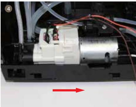
4. Move the dispenser valve group to the right side according to the direction of the arrow
