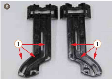
8. Install the left and right pull plate and left and right cover on brew unit frame, oil (MI-setral-61B) coating position for left and right pull plate should be as the picture shows.
