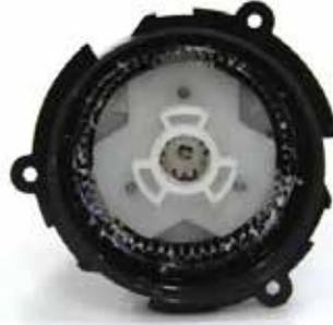
5. Put the already installed epicyclic gear frame B into gearbox.
