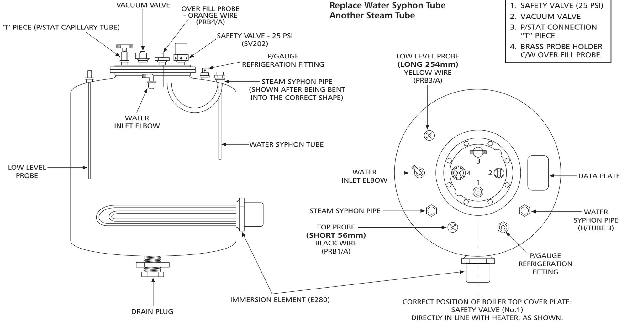
**IMPORTANT: ENSURE PROBES ARE IN THE CORRECT PLACE**
