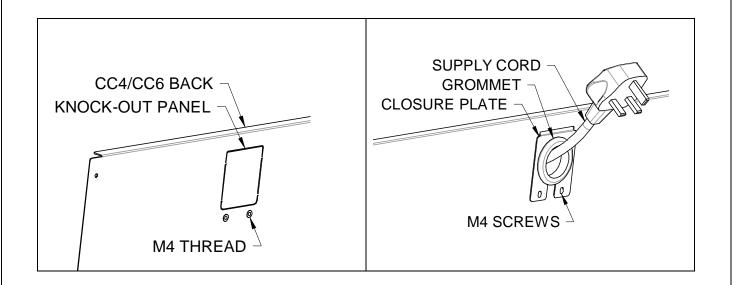
To fit SLI21, SLI3, SLI3W to the CC4 ambient pedestal, or the SLI42 to the CC6 ambient pedestal, the knock-out panel has to be removed.
