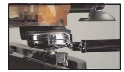
b) Pull the feeder handle (14) towards you to obtain a single measure. Release the handle for it to return to its position.
