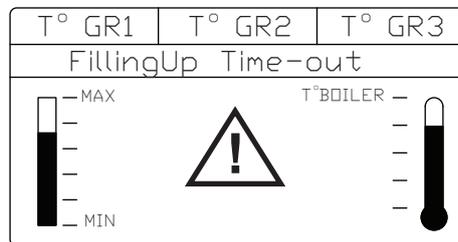
**CAUSE:** The water in the steam boiler has not reached the level probe in the set refilling time, after this will occur during initial start up, when the boiler is filling up from empty.
