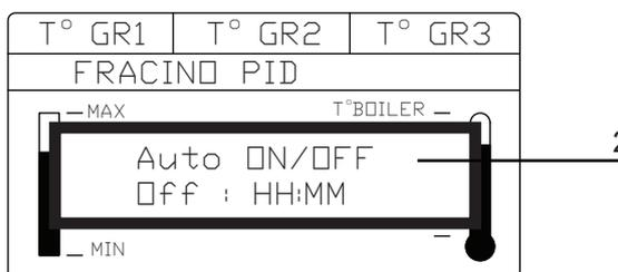
NOTE: When using the Auto on/off the machine will go into stand-by mode and will not isolate power from the machine.
