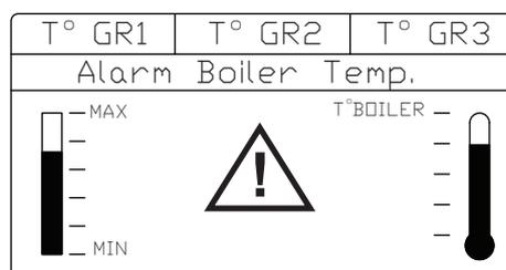
**CAUSE:** The temperature in the steam boiler has reached 140°C, and the heating element has been deactivated. To get to this temperature there is likely to be a fault with the Pressure switch and high limit thermostat.
