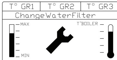
If the spanner symbol appears with the “Change Water Filter” in the Scroll menu the water filter needs to be replaced, contact Fracino or your local service agent to have the filter replaced.
