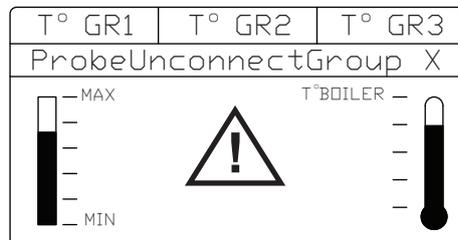
**CAUSE:** The temperature probe on group “X” has been disconnected or has developed a fault.
