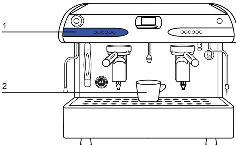
1. The duration of the hot water dispensing can be adjusted using the left hand key pad
