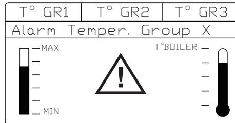
**CAUSE:** The temperature in group “X” has risen above 140° C, possibly caused by a fault in the group temperature probe and/or a fault with the group high limit thermostat.
