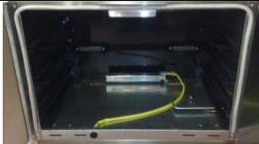
Unscrew the 15mm nut on the jet that goes into the burner
