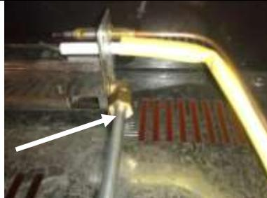
Unwind the jet out of the burner
