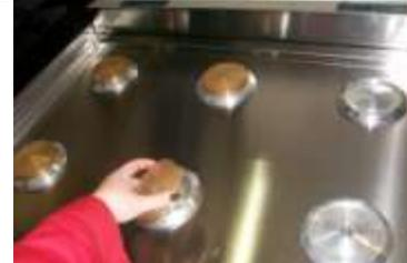
Lift off aluminium burner plates.
