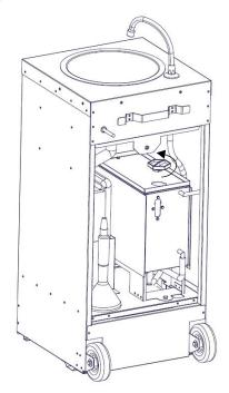
Once the rear panel has been removed, the hot water cap can be removed by twisting anti-clockwise. With the cap removed, the flexible plastic funnel supplied with the unit can be used to fill the tank up to the level shown on the fill level indicator on the tank. The filler cap can then be secured back in position.
