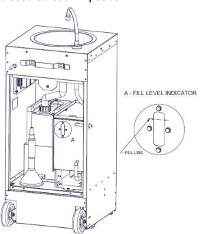
Power the unit up by connecting it to a suitable power source, the green light indicator on the front of the unit should light up once this is done. Once the unit has been connected, the element in the hot water tank will start heating up the water immediately; it should take approximately 15 minutes to reach operating temperature on a full tank of water.
