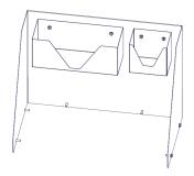
The splashback is simply fixed to the unit using six M5 screws which are supplied with the splashback when chosen as an optional extra. The figure below shows the height of the unit when the splashback is present.
