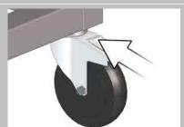
Release the transport trolley's parking brakes.
