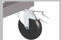
Release the transport trolley's parking brakes.
