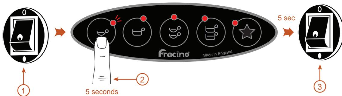
The machine is fitted with a pre-infusion feature, which puts a 1second on/off pre-infusion on to the single espresso and single coffee. The pre-infusion is activated in the following procedure:
