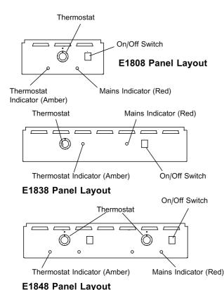
The ON/OFF switch controls power to the controls.
