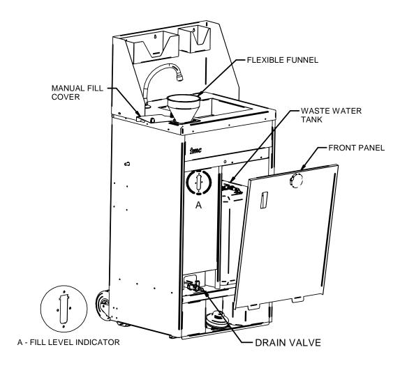
Power the unit up by connecting it to a suitable power source. Once the unit has been connected, the element in the hot water tank will start heating up the water immediately; it should take approximately 15 minutes to reach operating temperature on a full tank of water.
