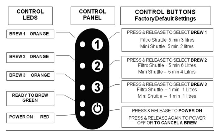
Note : Default settings may vary depending on local connection factors, if required recalibration can be carried see Setting Brew Water Volumes/Water Flow Times section.
