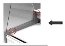
Place both side glasses and fix them to counter sides using screws as in picture
