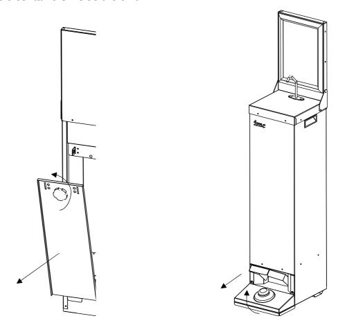
Once the rear panel has been removed, fit the suction hose pipe into the sanitiser container. Place the container on to the inner base panel. Note the suction tube is suitable for 5 litre containers.
